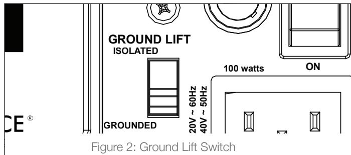
Figure 2: Ground Lift Switch
