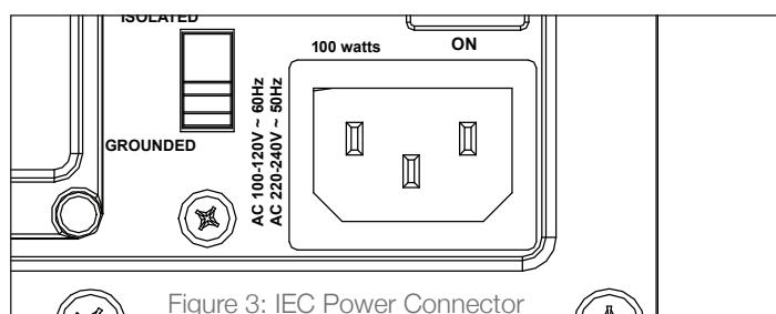
Figure 3: IEC Power Connector
