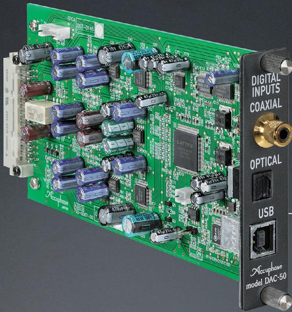
Digital Input Board With USB, Optical, and Coaxial Inputs
