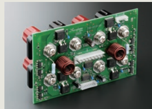
Protection circuitry with MOS-FET switches
