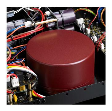
The heart of the HINT 6's power supply is a massive 1.1 kVA toroid power transformer. It is custom designed for well-contained radiated hum, high efficiency, and high power. Encapsulating this massive power transformer in an epoxy-filled steel canister assures ultra-quiet performance.
