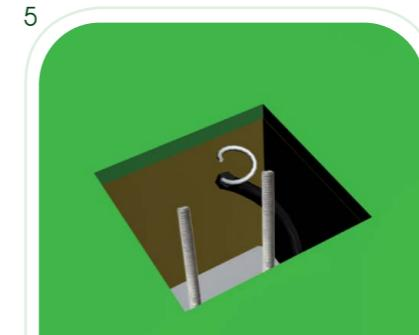
The point where the pipe comes out of the ground must be located at the center of the hole, with a view to ensuring the proper mounting of the upper plate.
