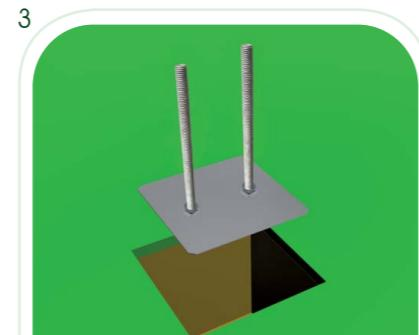
Lay the HRX031 bracket underground so that the upper ends of threaded rods stick out of the floor by about 12 mm once the hole has been filled.
