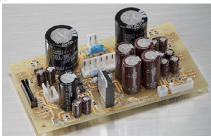
Pre-stage/drive stage power supply assembly
